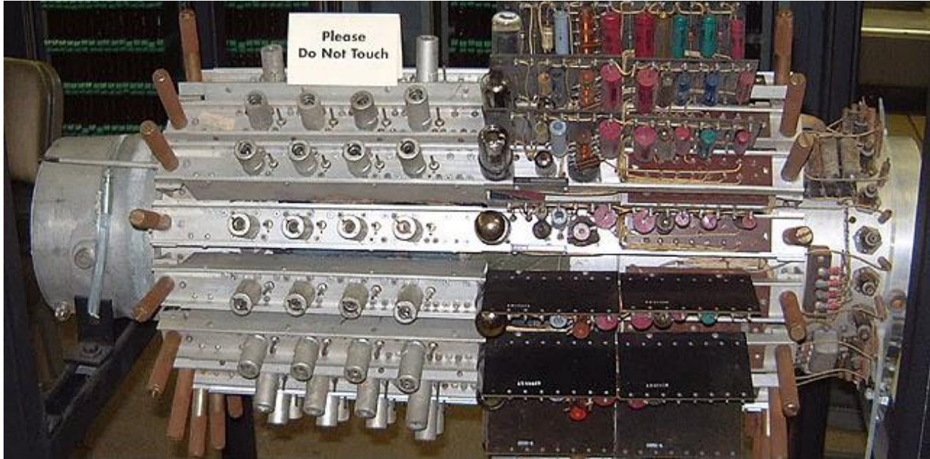
Mercury memory of UNIVAC I (1951) CC BY-SA 3.0, https://commons.wikimedia.org/w/index.php?curid=64409
